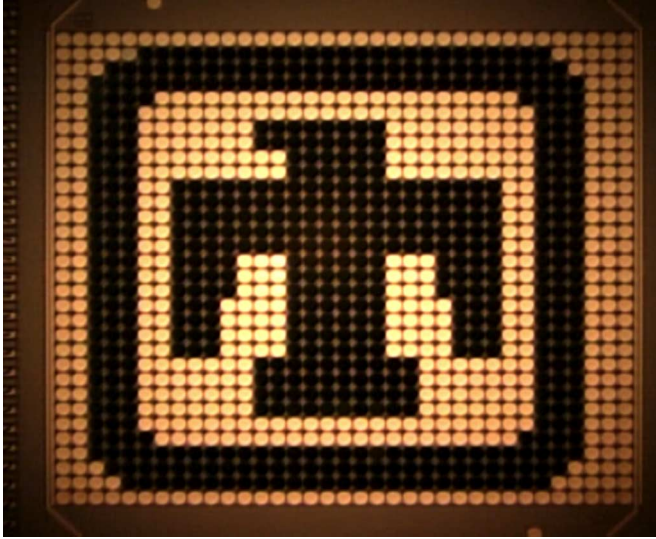
Fig. 6. MEMS is a 32 \times 35 array of 240 \mu\text{m} diameter mirrors.
